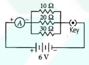
(a) Given: Voltage of the battery = 2V + 2V + 2V = 6VCurrent through  $10\Omega$  resistance:  $I_{10} = V/R = 6/10 = 0.6A$ Current through  $20\Omega$  resistance:  $I_{20} = V/R = 6/20 = 0.3A$ Current through  $30\Omega$  resistance:  $I_{30} = V/R = 6/30 = 0.2A$ (b) Total current in the circuit:  $I_{total} = I_{10} + I_{20} + I_{30}$  $I_{total} = 0.6 + 0.3 + 0.2 = 1.1A$ (c) Total resistance of the circuit:  $1/R_p = 1/10 + 1/20 + 1/30 = 11/60$  $R_p = 60/11 \approx 5.45\Omega$
