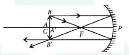
Ans11. (a) (i) Pole : The centre of the reflecting surface of a spherical mirror is a point called the pole. It lies in the surface of the mirror and its represented by the letter P.
