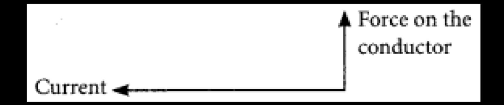
Using Fleming's left hand rule, the direction of magnetic field is out of the plane of paper.
